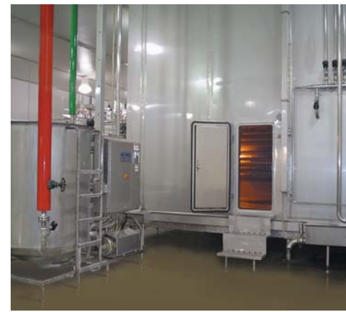
GEA A-Tec series recirculating CIP system
