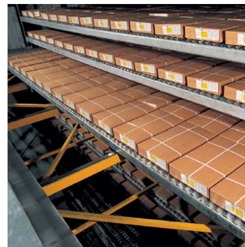
Raw chicken in boxes in a GEA I-VRT carton freezer
